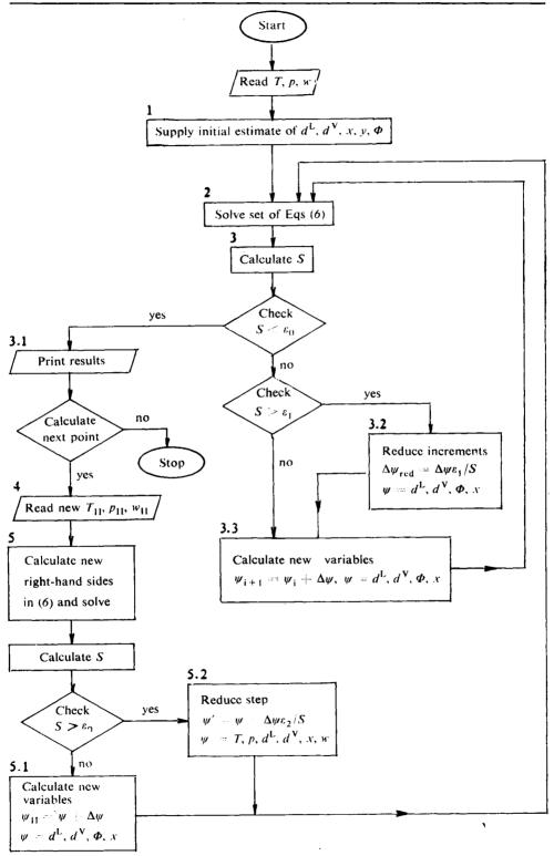
Thus the set of N + 2 equations with N + 2 unknowns  $d^{V}$ ,  $d^{L}$ ,  $\Phi$ , x is obtained. The flow diagram of the computational procedure is shown in Scheme 1 and entails the following steps:
